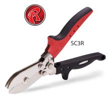
Ideal for crimping heavy 24 to 22 gauge (0.71 to 0.86 mm) galvanized sheet steel.
