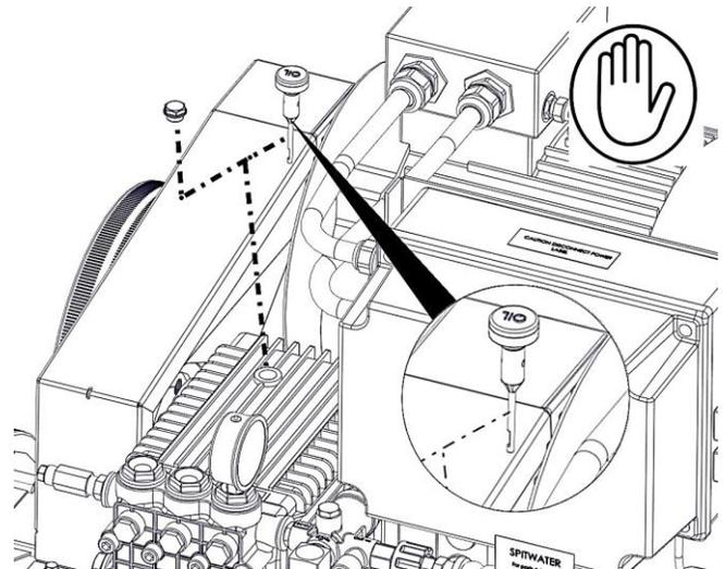
8. Check the oil level in the pump using the dipstick or the sight glass on the back / side of the pump. Make sure the level is between min/max level notches on the dipstick, or is level with the indicator on the sight glass. If oil reservoir needs replenishing only use oil of a type as listed in the data sheet in this instruction manual.
