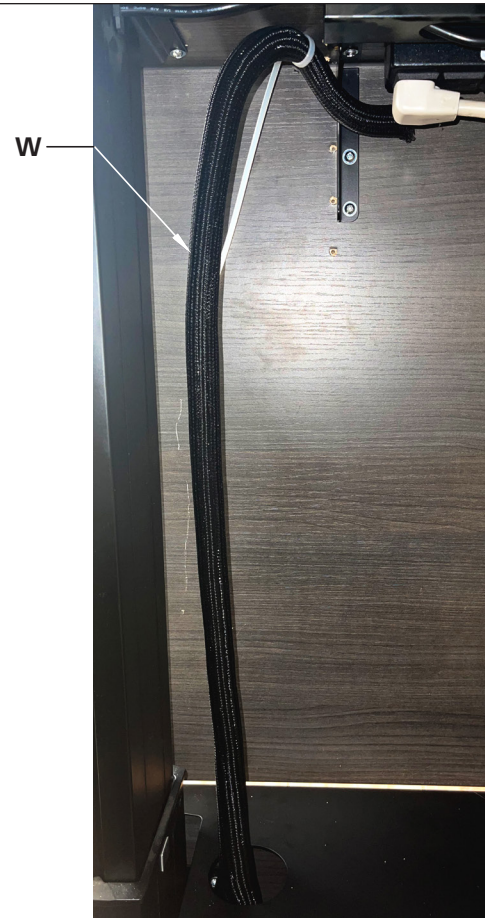
Showing the mesh cable sleeve wrapped around cords
