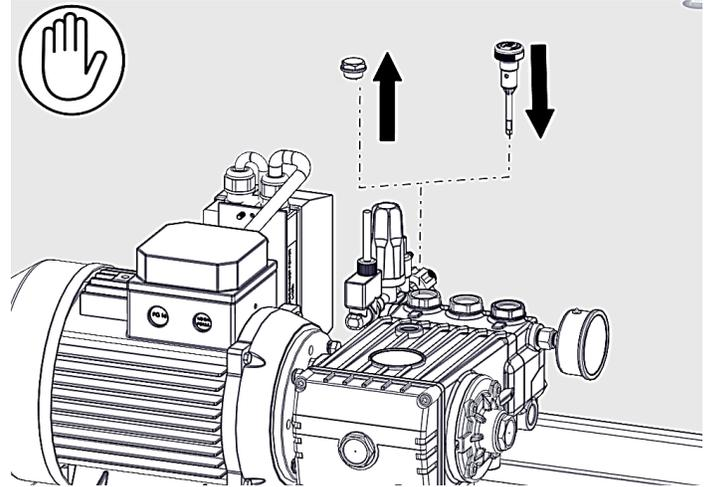
8. Check the oil level in the pump using the dipstick or the sight glass on the back / side of the pump. Make sure the level is between min/max level notches on the dipstick, or is level with the indicator on the sight glass. If oil reservoir needs replenishing only use oil of a type as listed in the data sheet in this instruction manual.
