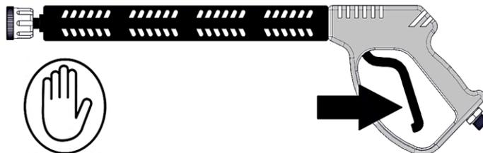
3. Check that the pressure indicated on the pressure gauge matches the value on the data plate and in the technical data. Also check that when the trigger is released the pressure shown on the gauge returns to zero.
