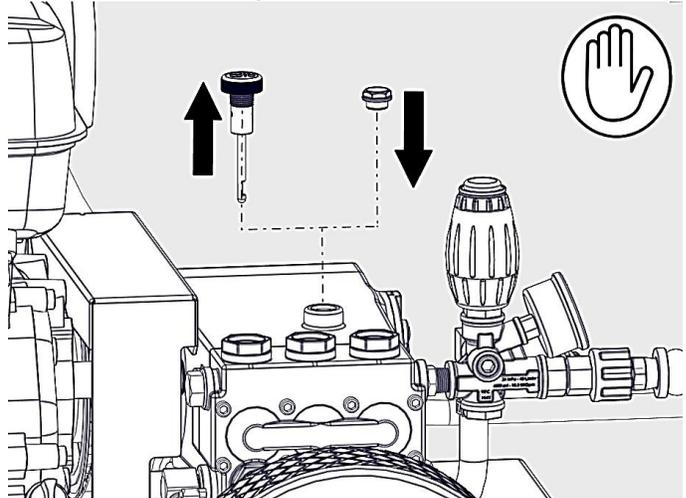
7. Check the oil level in the pump using the dipstick or the sight glass on the back / side of the pump. Make sure the level is between min/max level notches on the dipstick, or is level with the indicator on the sight glass. If oil reservoir needs replenishing only use oil of a type as listed in the data sheet in this instruction manual.
