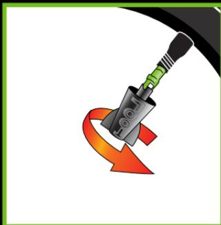
**6** Reinstall valve core.
