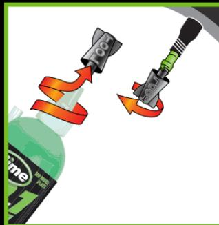
**3** Slowly remove valve core with tool in cap.
