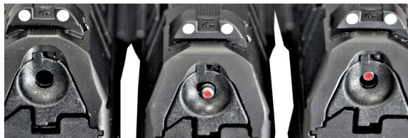
3.2.2. Fig. 1, from left to right: de-cocked, cocked, cocked (P99 QA only)
