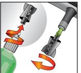
Slowly remove valve core with tool in cap.
