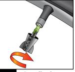
Reinstall valve core.
