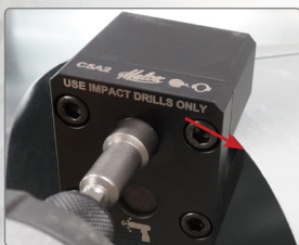
Begin crimping at angle after crease
