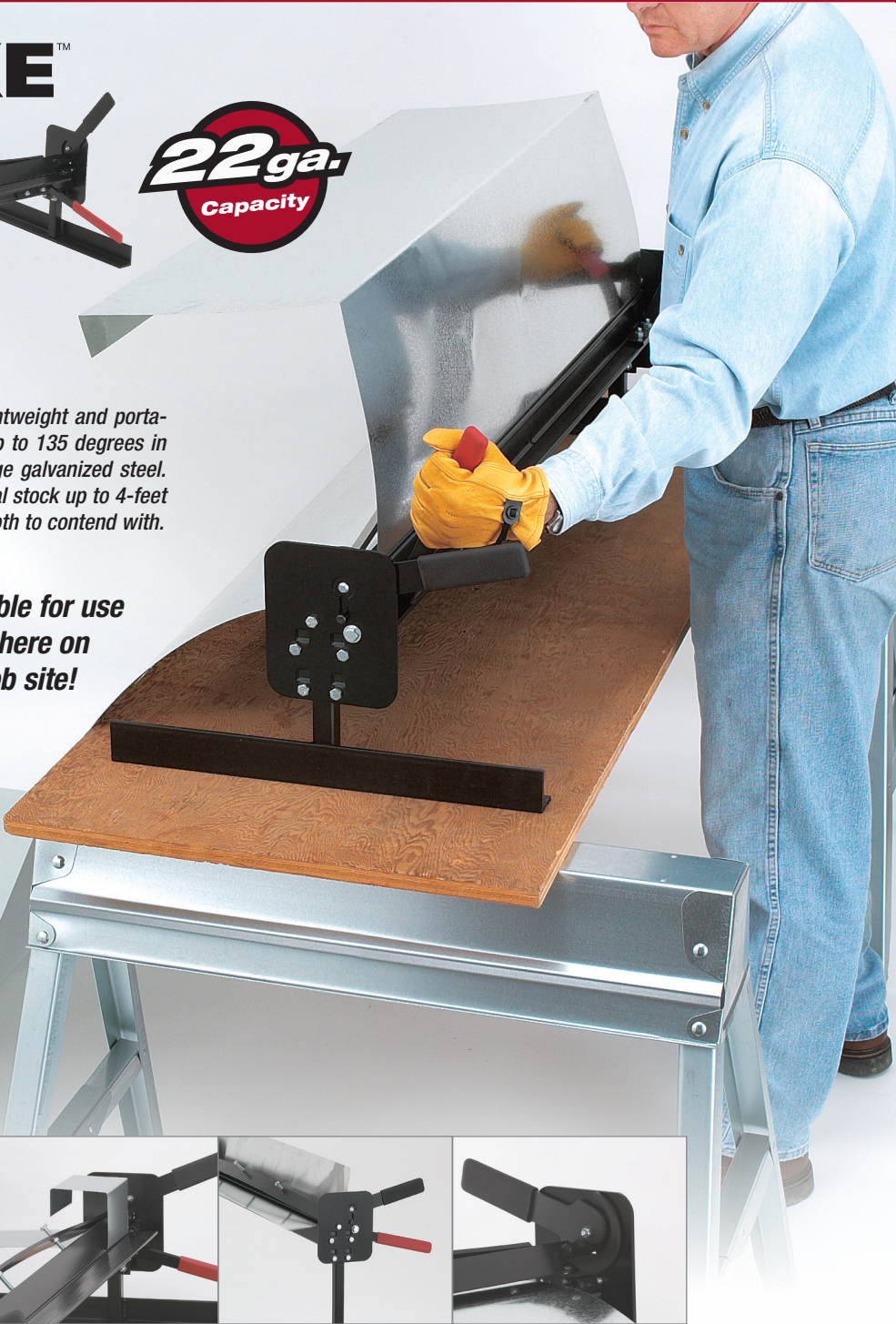
Versatile bending range accommodates compact fabrications as small as a 4-in. (101.6 mm) square.
