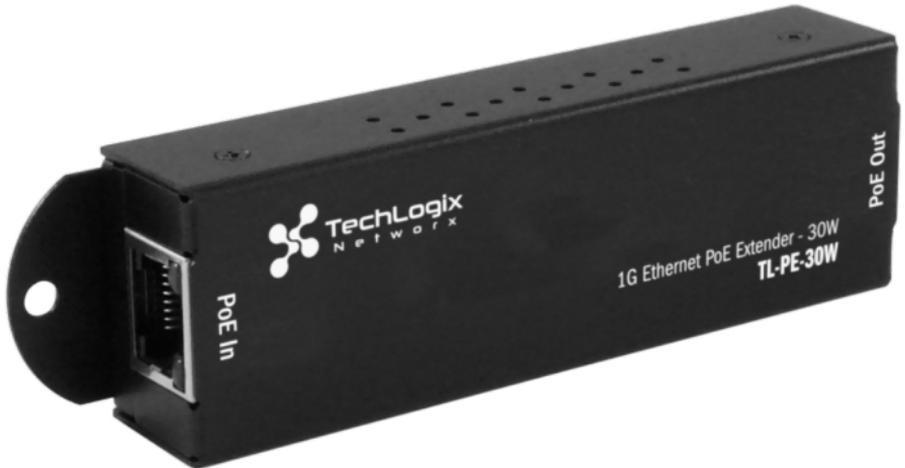
The TechLogix Network TL-PE-30W is designed to extend connection distances from a PoE source to an output device another 100 m (328 ft.) via twisted pair cable. You can cover even longer distances by cascading these extenders on a network. The TL-PE-30W does not need any additional power supply, as it draws the power it needs from the PoE input.
