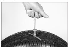
With the plug centered in the eye of the needle, start pushing the plugger tool and plug into your puncture. The insertion tool collar will stop the insertion of the plug at a certain depth to help ensure the plug is inserted to the proper depth.
