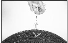
Pull the plugger tool straight out of your tire with a rapid motion, leaving the tire plug behind. Do not twist the needle.
