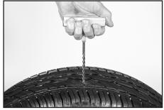
Slide the reamer tool in and out of your Remove a plug from its clear backing, tire puncture multiple times to roughen then thread it halfway through the eye and clean the inside of the hole.
