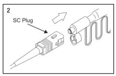
Insert SC connector onto the Guide Cap.
