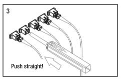
Push the Outer Shell to start cleaning the SC connector end face. A "click" sound indicates end of cleaning process. Close the cover after use.
