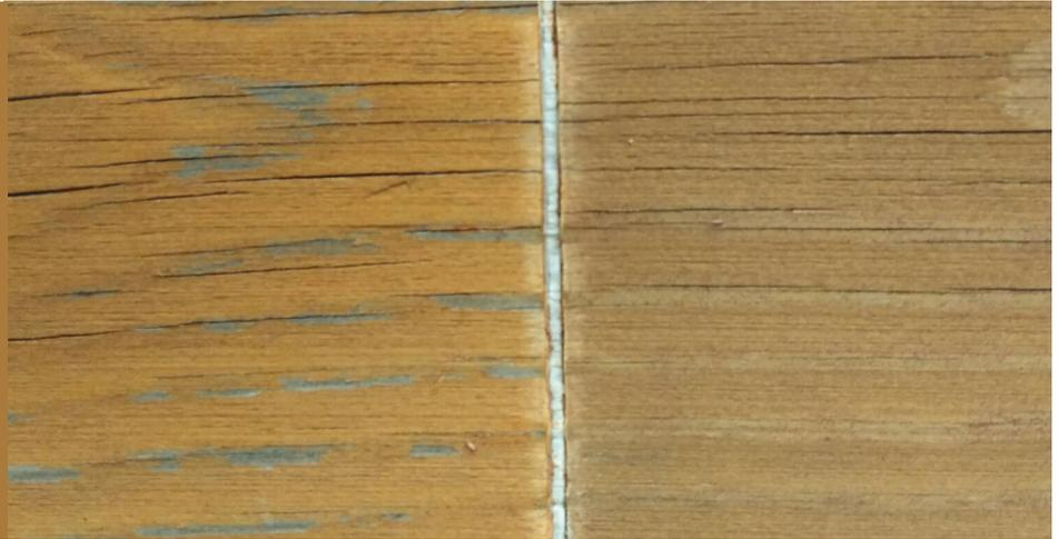
**Hard Acrylic vs. Elastic Acrylic** An unusually hard acrylic stain alongside Capture® with Cascade® on the right. Both were exposed for 18 months. The hard acrylic cracked and peeled profusely. Breathability hardly matters for that stain. On the Capture® side, there is nearly no damage because it kept water out. Even where there are cracks in the wood, peeling has not started yet because Capture® and Cascade® are still very breathable.
