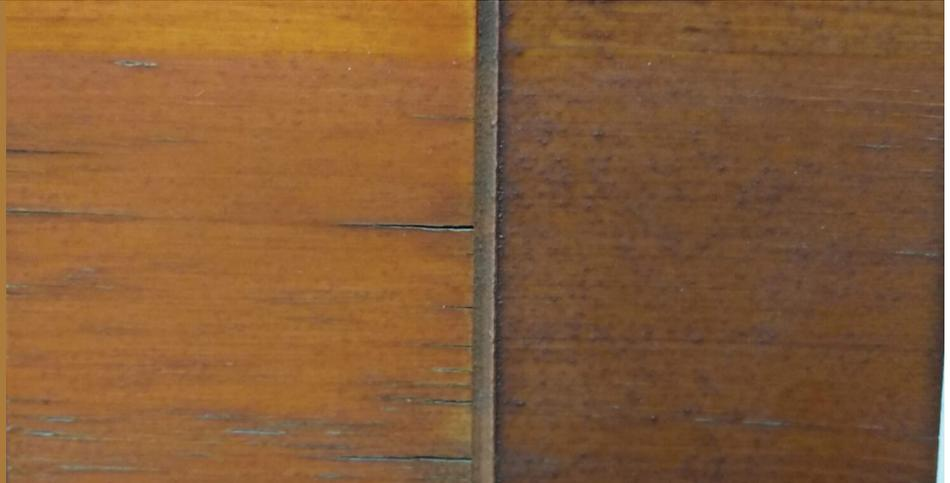
**Non-drying oil vs. Flexible Drying Oil** *This panel shows a non-drying oil stain (left) vs. Transformation Stain® Log and Timber (right) after 24 months exposure. Although the non-drying oils have superb breathability, they simply don't last, and as mentioned earlier, will keep sealants (and some future stains) from adhering properly.*
