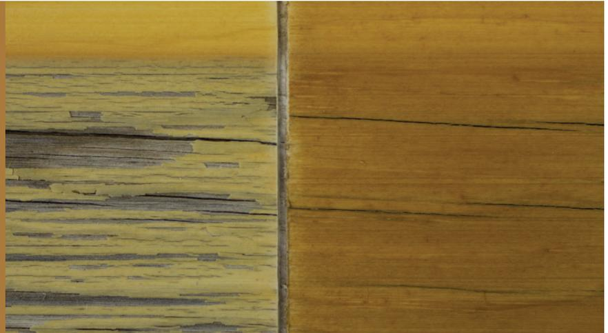
**Typical Acrylic** Here we see a common acrylic stain versus Sashco's Capture® and Cascade® stain system, exposed for 18 months. Note that on the left, the water getting into the wood has cracked and aged the wood, as well as the stain, but on the right side, with hyperelastic Capture®, the stain is still looking very good.
