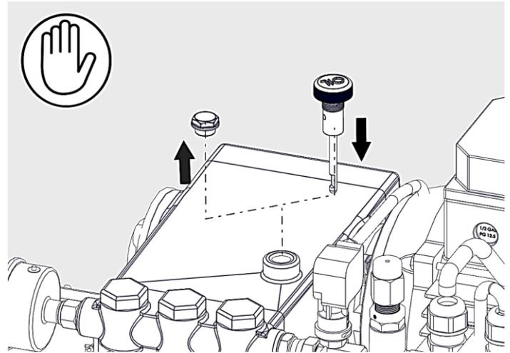
9. Check the oil level in the pump using the dipstick or the sight glass on the back / side of the pump. Make sure the level is between min/max level notches on the dipstick, or is level with the indicator on the sight glass. If oil reservoir needs replenishing only use oil of a type as listed in the data sheet in this instruction manual.
