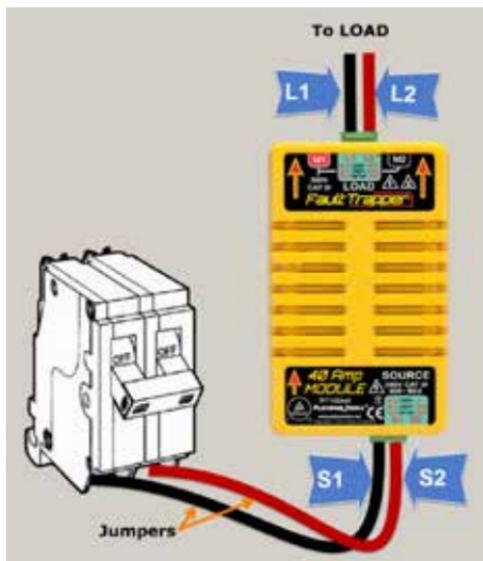
1. Remove the two hot wires from the breakers for the load being tested and attach them to the Load side of the Fault Trapper 40A In-Line Adapter Module with the black in Load Terminal “L1” and the red wire in Load Terminal “L2” using the Plug-in Terminal Block Connector.
