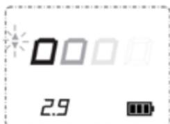
Testing for 2.9 min, no faults
