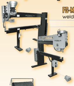
FE-Mach 70 & RH Mach 70 Automatic Physiothers® for welded insulation fastening.
