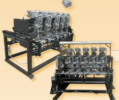
FEMALE PLESPONERS® FGMH for welded insulation fastening and HSMH - High Speed Multihead Pinspotter® capable of welding up to 2 inch pins on 16 gauge material as close as 6 inch centers at speeds of 50+ feet per minute.
