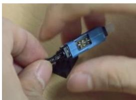
Remove the connector jig
