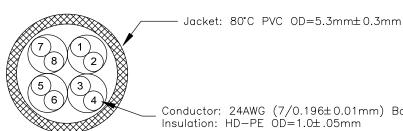
Conductor: 24AWG (7/0.196±0.01mm) Bare copper
