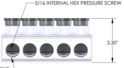
**WIRE ENTRY POINT** WIRE RANGE: 500MCM - #4AWG PRE-FILLED W/ OXIDE INHIBITOR
