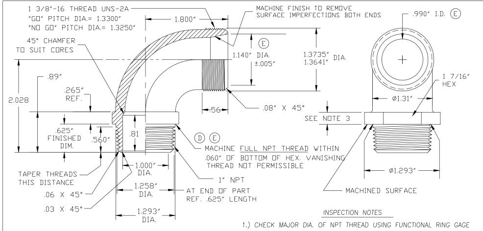
(.135" THK. X 1.265" I.D.) PLACE GAGE OVER NPT THREAD. GAGE SHOULD FIT APPROX FLUSH WITH END OF PART BUT NOT BEYOND
