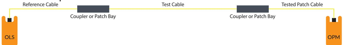
**Alternate Test Setup**
