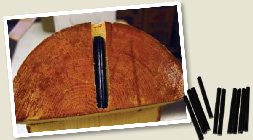
Log cross-section showing an installed borate rod.
