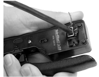
Insert connector into the Tele-Titan XG 2.0 crimp tool and compress the handle. The contacts are terminated.
