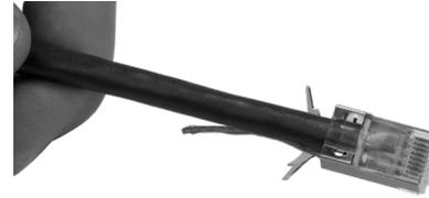
Insert assembly into connector and ensure conductors pass all the way to the front end of the connector. Verify by looking into front end.
