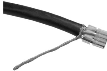
Slide the load bar/liner all the way down flush to the pair spacer bar and trim conductors flush against the load bar/liner front end using the 5" Side cutting Pliers, P/N 10531C.
