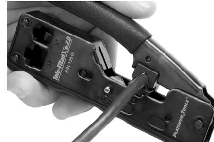
Grounding can be done using foil, braid, or a drain wire. Use the rear cavity of the Tele-Titan XG 2.0 to crimp external ground tab onto cable, securing the ground.
