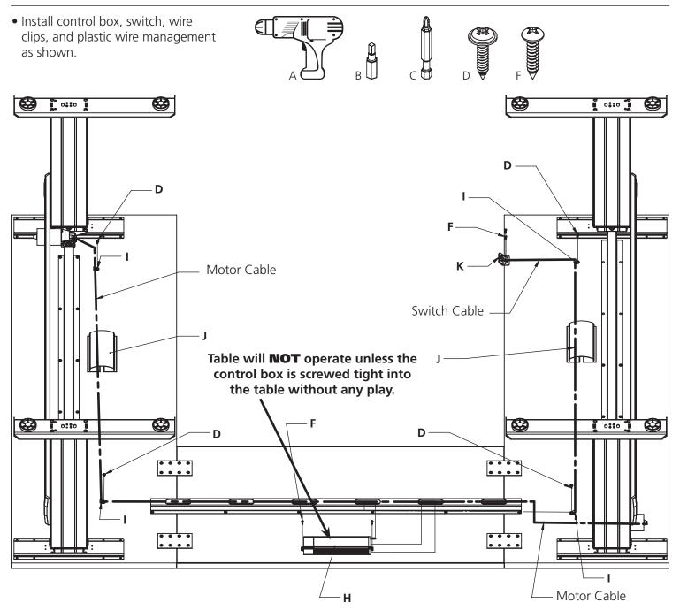
**Caution:** For the safety of the user and the workstation; the control box contains an internal sensor that is sensitive to movement, vibration, and collision. For faultless operation, ensure
