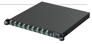
Power Supply Unit (PSU) functionality is integrated into the Secondary Hub chassis and powers the Remotes via 48V DC, available on eight 2-way Phoenix connectors (which connect to the attached Remotes via copper wire). Secondary Hubs can be housed with the Primary Hub or distributed campus-wide, depending on the site layout.
