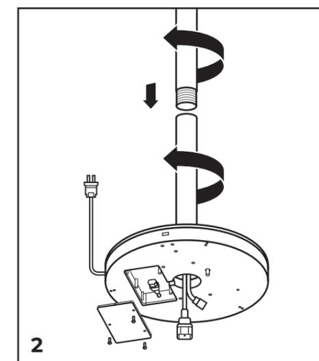
2 Thread the bottom pole into the base. Next, thread the middle pole into the bottom pole.
