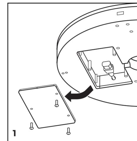
1 Remove the wiring compartment cover.
