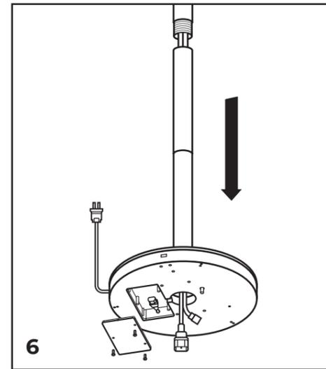
6 Feed the LED and power cables through the middle pole, bottom pole, and base of the unit. Screw the top pole into the middle pole.
