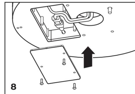
8 Re-install the wiring compartment cover.
