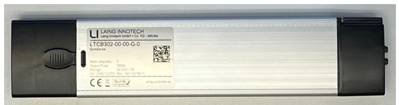
Battery pack inserted into control box housing
