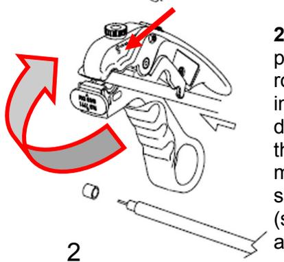
2. For best performance, rotate stripper in same direction as the arrow molded on side of tool (see red arrow)
