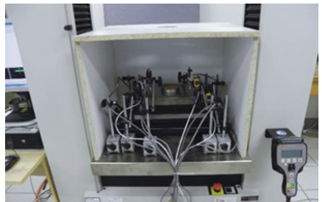
Figure 4: Test setup used for elevated temperature compression test
