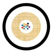
*S2I-12M-P-BK* fiber optic cable is constructed with twelve internal tight buffers, internal aramid yarn, and one outer plenum-rated PVC jacket in distribution format. The fiber cable features a water-resistant jacket and is designed for indoor and outdoor applications.
