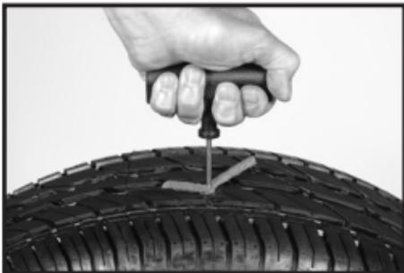
Push the plugger tool and plug into your puncture. Stop pushing when the plug is 2/3 of the way into the hole.
