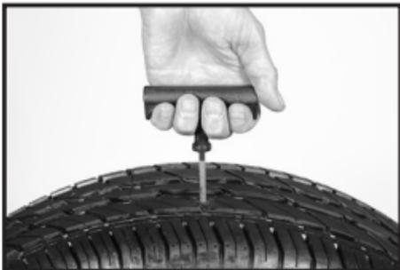
Slide the reamer tool in and out of your tire puncture multiple times to roughen and clean the inside of the hole.
