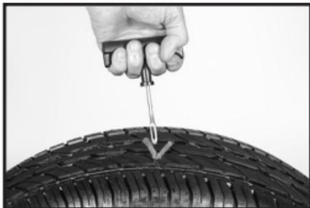
Pull the plugger tool straight out of your tire with a rapid motion, leaving the tire plug behind. Do not twist the needle.
