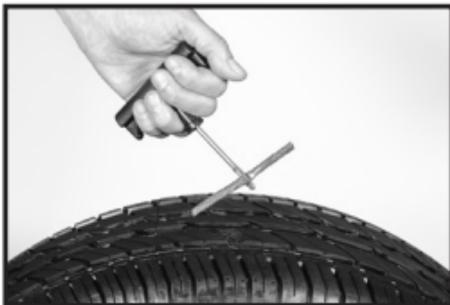
Remove a plug from its clear backing, then thread it halfway through the eye of the plugger needle.
