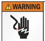
**Electrical Shock Hazard** Disconnect power before servicing Replace all parts and panels before reconnecting power.
