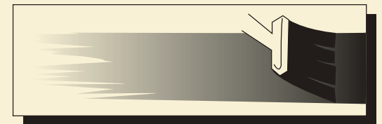
Feathering Technique: use only if stopping in the middle of a wall is unavoidable.
