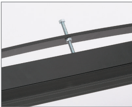
A 5/16 in. (7.9 mm) plate steel apron & adjustable strengthening ribs on anvil assure uniform bends across width of material.
