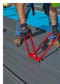
FSHS2 Works on 2" vertical seams with 13/16" width
