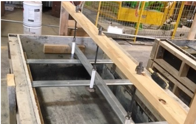
Figure 5 – RapidBrace PT Duct testing setup
