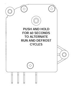
Some refrigerators do not use plug-in connectors for a defrost timer hook-up. Each terminal is connected using a seperate wire. In this case, very carefully bend terminals 2, 4, 3 as illustrated. Use needle-nose plier to hold the terminal while bending it with another plier.
