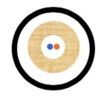
*M4I-2M-P-BK* fiber optic cable is constructed with two internal tight buffers, internal aramid yarn, and one outer plenum-rated PVC jacket in 900µm distribution format. The cable features a water-resistant jacket and is designed for indoor and outdoor applications.
