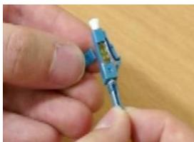
Remove the connector jig
