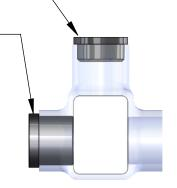
WIRE ENTRY POINT WIRE RANGE: 600MCM - #6AWG PRE-FILLED W/ OXIDE INHIBITOR-
