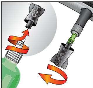
**2** Slowly remove valve core with tool in cap.
