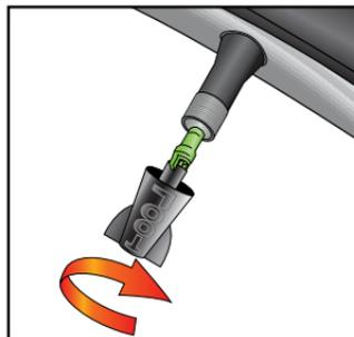
**6** Reinstall valve core.
