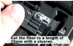
**Cut the fiber to a length of 10mm with a cleaver.**
