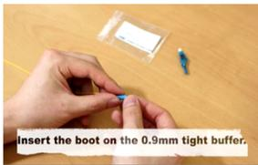
**Insert the boot on the 0.9mm tight buffer.**
