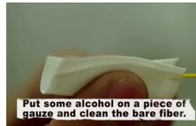
**Put some alcohol on a piece of gauze and clean the bare fiber.**
