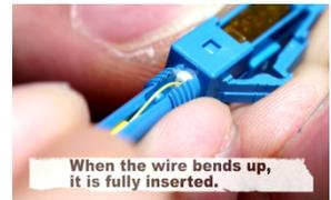
**When the wire bends up, it is fully inserted.**
