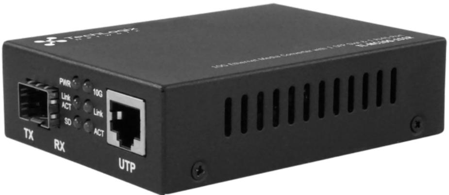
The TL-MC10G-1S1R features one SFP+ port (SFP module sold separately) and one RJ45 twisted pair port, effectively adapting twisted pair-based devices to fiber for longer transmission distances. The TL-MC10G-1S1R supports multimode fiber when paired with a multimode SFP+ module and single mode fiber when paired with a single mode SFP+ module.
