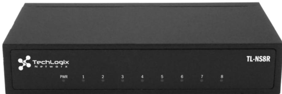
The TL-NS8R includes eight Gigabit Ethernet ports, providing you with high performance on your network to handle quick transfer speeds that support disk mirroring, data backup, graphics image file transfers and other bandwidth-intensive applications.
