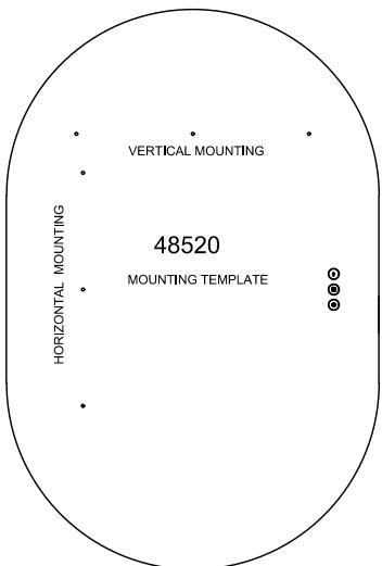
Temporarily secure the paper (G) to the wall, then mark the anchor (D) locations on the wall through the holes. Remove the paper (G) and drill holes making them slightly smaller than the anchors (D) provided.
