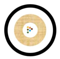
*M4I-6M-P* fiber optic cable is constructed with six fiber strands, internal aramid yarn, and one outer plenum-rated PVC jacket in distribution format. The cable features a water-resistant jacket and is designed for indoor and outdoor applications.
