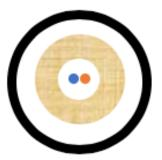
*S2I-2M-P-BK* fiber optic cable is constructed with two internal tight buffers, internal aramid yarn, and one outer plenum-rated PVC jacket in distribution format. The fiber cable features a water-resistant jacket and is designed for indoor and outdoor applications.
