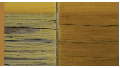
**Typical Acrylic** Here we see a common acrylic stain versus Sashco's Capture® and Cascade® stain system, exposed for 18 months. Note that on the left, the water getting into the wood has cracked and aged the wood, as well as the stain, but on the right side, with hyperelastic Capture®, the stain is still looking very good.
