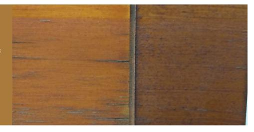
Non-drying oil vs. Flexible Drying Oil This panel shows a non-drying oil stain (left) vs. Transformation Stain® Log and Timber (right) after 24 months exposure. Although the non-drying oils have superb breathability, they simply don't last, and as mentioned earlier, will keep sealants (and some future stains) from adhering properly.
