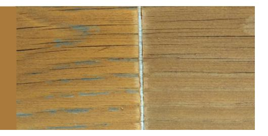
Hard Acrylic vs. Elastic Acrylic An unusually hard acrylic stain alongside Capture® with Cascade® on the right. Both were exposed for 18 months. The hard acrylic cracked and peeled profusely. Breathability hardly matters for that stain. On the Capture® side, there is nearly no damage because it kept water out. Even where there are cracks in the wood, peeling has not started yet because Capture® and Cascade® are still very breathable.
