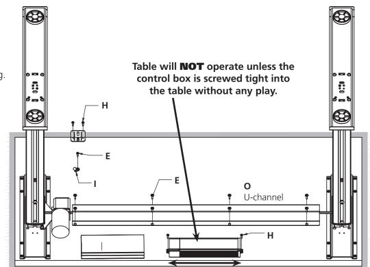
**Control Box Orientation must be mounted this way**
