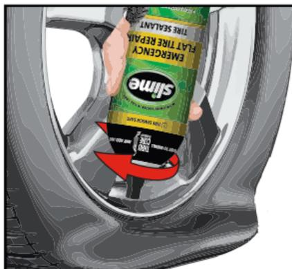
**3** Turn can upside down and screw plastic nozzle clockwise onto tire valve.
