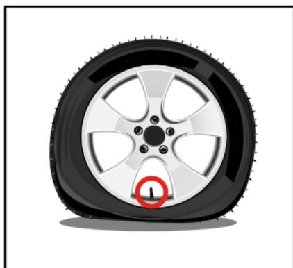
**1** Position valve at 6 o'clock on tire.
