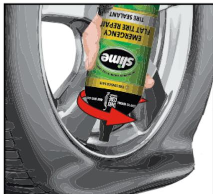
**4** Allow 30 seconds for can to discharge fully. Unscrew nozzle when empty.
