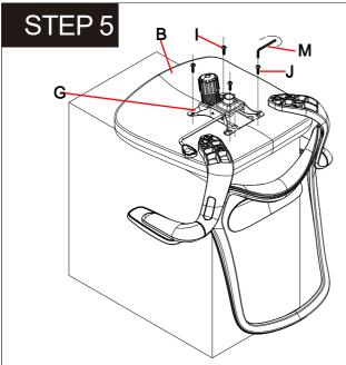
Use the correct Mechanism Bolts (J) and Back Bolts (I), Assemble the Mechanism (G) to the Seat Cushion (B), using 2 Mechanism Bolts (J) and 2 Back Bolts (I), Tighten the bolts securely with the Allen Wrench (M).
