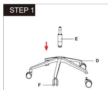
Press the Casters (F) into the holes at the end of each leg of the Base (D). Inset Seat Post (E) into the center hole of the Base.
