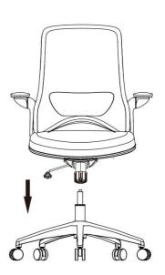
Now turn the assembled seat upright and locate the center hole of the Mechanism over the Seat Post. Push down firmly until the connection is secure.
