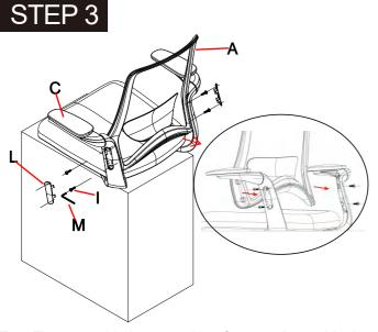
Turn The assembled seat cushion face up, Assemble the Backrest (A) to the Armrest (C), Using 4 Back Bolts (I), Tighten the bolts securely with the Allen Wrench (M). Assembled the small cover (L) to the Armrest.
