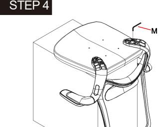
After the backrest assembly is completed, Tighten the Armrest bolts securely with the Allen Wrench (M).
